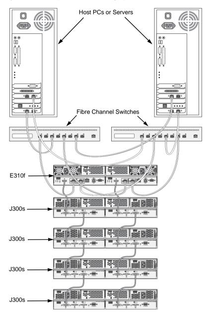
Figure 14. JBOD expansion with no single point of failure
